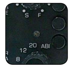
Note: only slight adjustments will be necessary, and should be made slowly, allowing the meter to settle between adjustments.. If the meter cannot be satisfactorily adjusted, it may be necessary to send the unit to the factory for a full calibration. *Contact BAE for service.*
